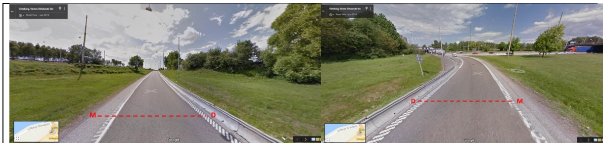
Figure 2.3 Images of the main remote sensing measurement site at Gullbergsmotet in 2016. The red dotted line and letters show the approximate position of the RSD instrument (D = source/detector, M = reflecting mirror). The left image is taken upstream, and the right image downstream of the RSD. The kerbside barrier on the right hand side was not in place in the 2016 measurements (images are from Google Maps 2014).
