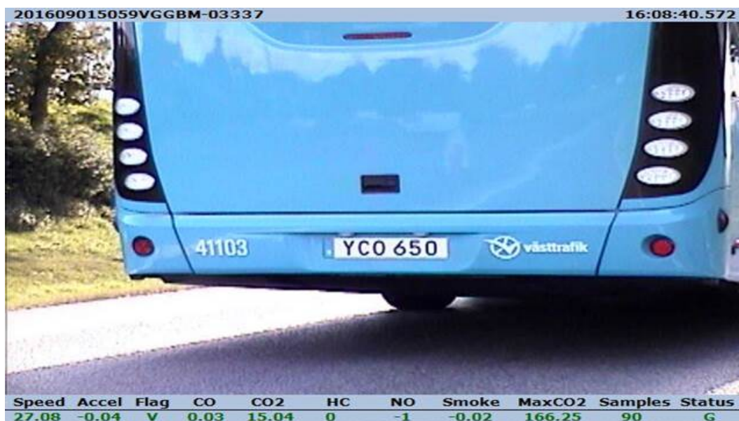
Figure 2.2 Image of the rear of the vehicle and the license plate as stored in the RSD 5000 instrument.
