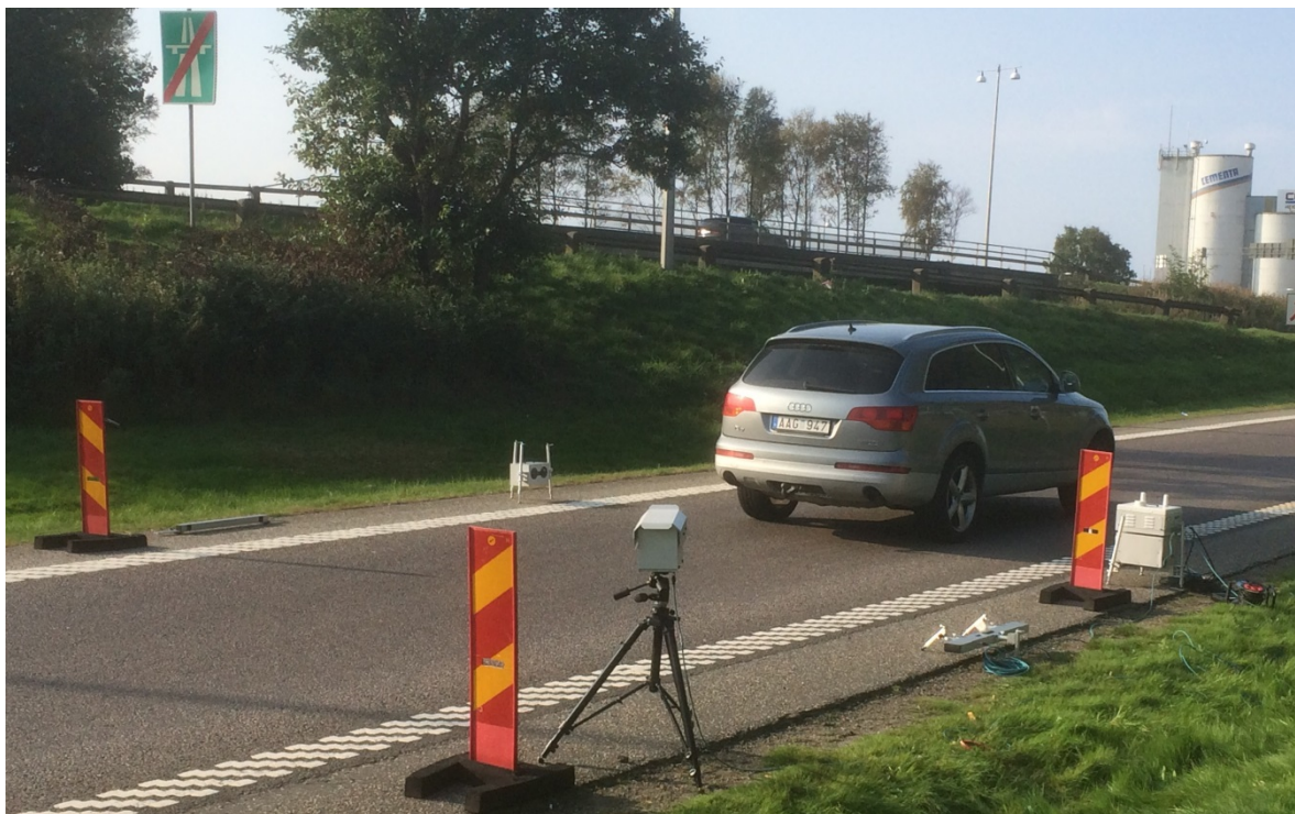
Figure 2.4 Set-up of the remote sensor at Gullbergsmotet.
