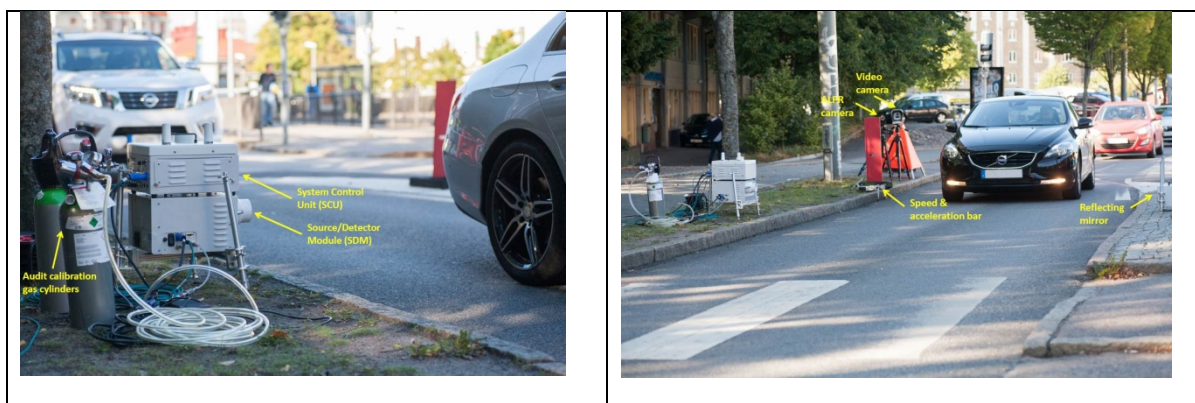
Figure 2.1 The new Opus AccuScan™ RSD 5000 instrument with NO 2 capability in operation in a city street in Gothenburg in September 2016. Pictures are copyright Opus.
